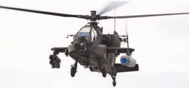
A high-energy laser system is shown above mounted on a U.S. Army Boeing AH-64 Apache attack helicopter during flight tests at White Sands Missile Range, N.M.
