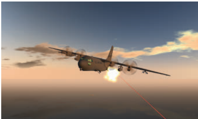
U.S. Special Operations Command is integrating a 60-kilowatt laser weapon aboard the AC-130J Ghosthunter gunship for air-to-ground interdiction.
