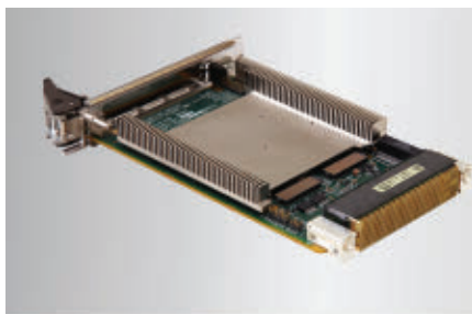
Curtiss-Wright Defense Solutions supports Green Hills Software's field-proven INTEGRITY-178 tuMP safety- and security-critical multicore RTOS on its VPX3-133 single board computer.
