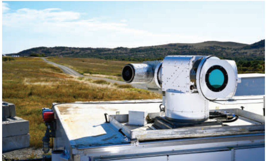
The Lockheed Martin Advanced Tactical High Energy Asset (ATHENA) is a prototype laser weapon system to defeat close-in, low-value threats such as improvised rockets, unmanned aerial systems, vehicles, and small boats.
