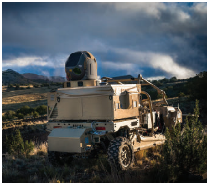
The Raytheon High Energy Laser Weapon System (HELWS) is shown mounted on a Polaris MRZR all-terrain vehicle. The laser uses pure energy to detect, identify, and take down enemy drones.
