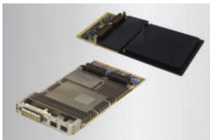
RTOS drivers are available for the Wind River VxWorks and Green Hills INTEGRITY-178 tuMP operating environments on Curtiss-Wright's XMC-4740 rugged video-processing mezzanine module.
