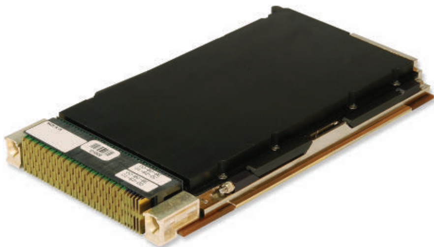
The Abaco 3U VPX SBC3511 provides SR-IOV capabilities in the data plane because it leverages the XL710 chipset.
